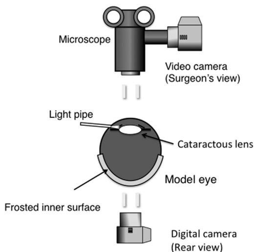
**Figure 2.** Schematic diagram of the experimental setup of the model eye. The images projected on the frosted posterior surface of the model eye (rear view) are recorded from the rear by a commercial digital camera. The images seen through the surgical microscope (surgeon's view) are also recorded by the video camera attached to the microscope.
